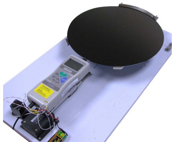
Figure 1. Test apparatus for measuring lateral holding force
